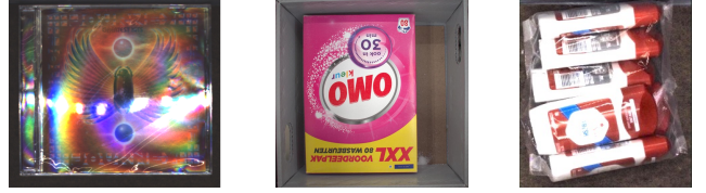
Figure 3. Examples for challenging defective cases (from left to right). (1) Unobservable cases. A small stripe in the bottom half of the CD could be either a reflection or a crack in the cover. (2) Complex cases. The detergent pack looks intact, but at a second look the powder on the tray next to it item indicates a spillage defect. (3) Ambiguous cases. The multi-pack is complete but its units are unordered, which is acceptable but has different visual appearance than the corresponding reference image.
