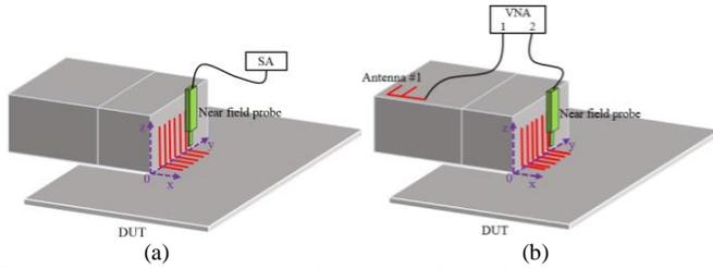
Fig. 3. (a) Measurement setup for near H field of forward problem. (b) Measurement setup for near H field of reverse problem.
