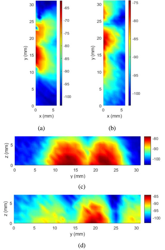
Fig. 4. Measured H field in forward problem. (a)  $H_x$  in  $x$ - $y$  plane at  $z=1$ mm. (b)  $H_y$  in  $x$ - $y$  plane at  $z=1$ mm. (c)  $H_x$  in  $y$ - $z$  plane at  $x=4$ mm. (d)  $H_y$  in  $y$ - $z$  plane at  $x=4$ mm.
