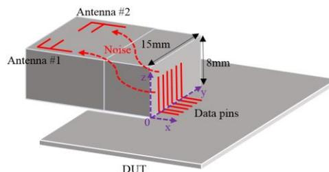
Fig. 1. Simplified description of the DUT.
