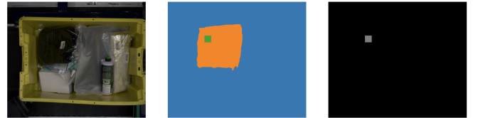
Fig. 11: Left: RGB input image. Middle: pick location and target item mask for our reference. Right: the pick location image which is used as an additional input.
