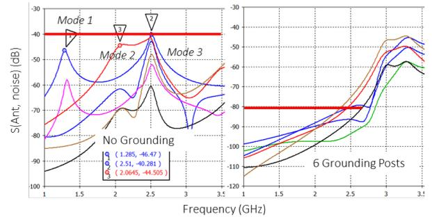
Fig. 1. Improvement of the noise to antenna coupling. No grounding posts has -40 coupling, peaks align with resonance frequencies. For 6 grounding posts, resonances are pushed to higher than 2.5 GHz, maximum coupling is ~ -80 dB at 2.5 GHz.
