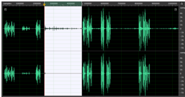
Figure 7 Waveforms of “NLEC=off” (top) and “NLEC=on” (bottom)
