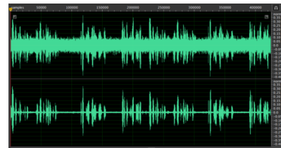
Figure 4 Waveforms of “before” (top) and “after” (bottom) SBNR Processing
